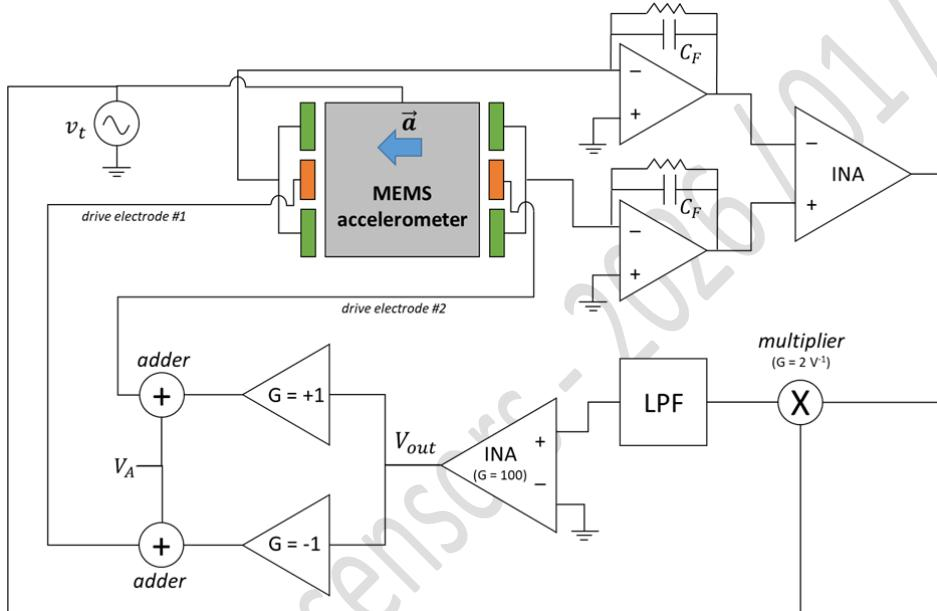
We see that part of the electronics (the rotor modulation voltage, the pair of charge amplifiers, the INA and the demodulation stage with multiplier and low-pass filter) is common to the classic circuit based on rotor modulation.
