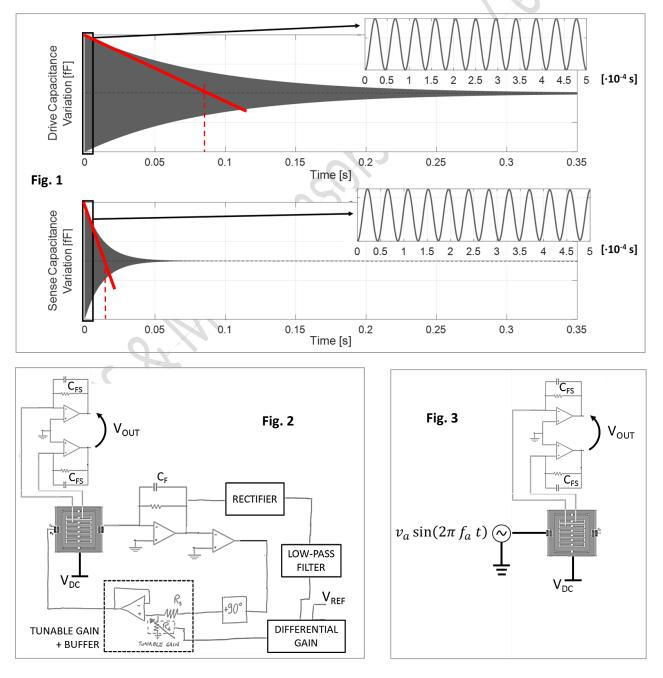
From the ringdown graph of each mode we can derive the resonance frequency and the quality factor. For the frequency, the relevant information is that appearing in the zoomed part of the image, where we find 11 periods in 500  $\mu$ s for the drive mode, and 11.5 periods in the same time for the sense mode. This gives us a resonant frequency of
