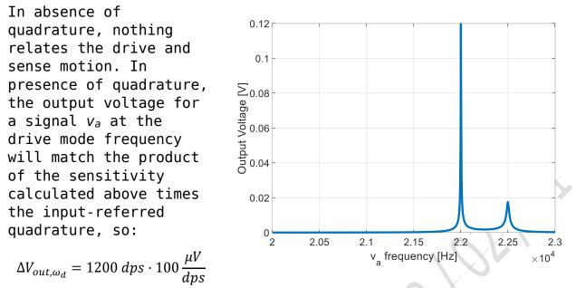
When moving forward in frequency the signal  $v_a$ , we pass also through the sense frequency. Here the drive motion will be lower with respect to the case above by a factor equal to  $Q_{eff}/Q_d$ . However, the quadrature force will be now amplified by the full Q factor of the sense mode, and thus increased by a factor  $Q_s/Q_{eff}$ . As a consequence, the output voltage can be easily quantified as the voltage calculated above, multiplied by a factor  $Q_s/Q_d$ .:
